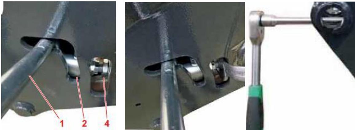
To set the lock, you will need an open-ended spanner (WAF 30), a ½" ratchet with the corresponding extension and 30 mm socket spanner.
