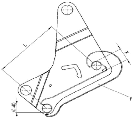
On the drive-in hook, check the front carriage of the 40 mm shaft and the hook (dimension of X max 63.2 mm). The hook is supplied as a weld-on part as a spare part.
