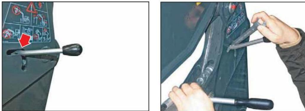
To set the lock, you will need an open-ended spanner (WAF 24), a ½" ratchet with the corresponding extension, joint and 24 mm socket spanner.
