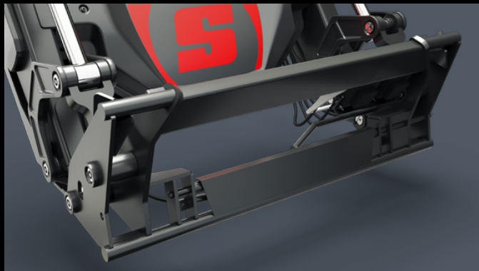
HYDRO-LOCK. Implement locking mechanism at the touch of a button, making it even more convenient to change the implement without having to get out of the cab.
