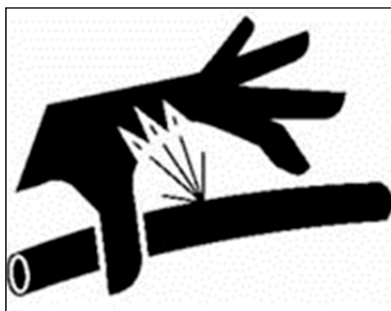
Figure 4: Risk of injury from leaking hydraulic oil.
