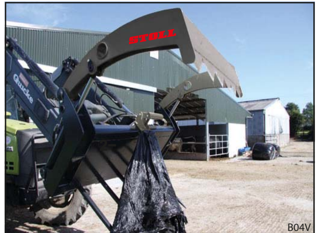
Fig. 42 Unloading the plastic wrapping
