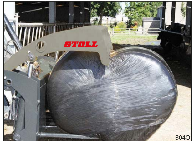
Fig. 37 Pressing the round bales against the main frame
